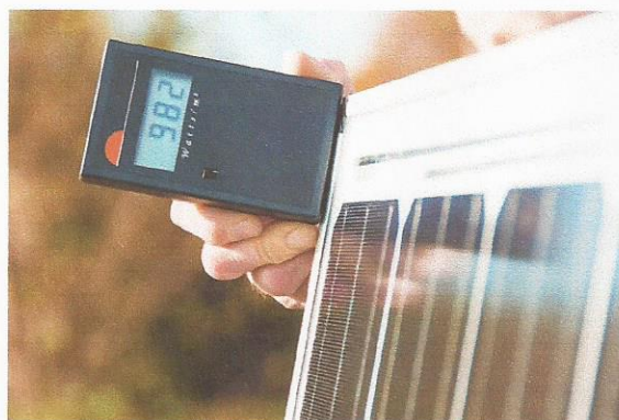
Figure C.8: Hand held solar meter measuring strong sunlight (982 Watts/m 2 ). The simultaneous solar module current was measured as 5.08 amps (Isc). This is acceptable because 5.08 amps (Isc) is nearly equal to the 5.11 amps (Isc) reported on the solar module specification (measured at standard test condition solar radiation of 1000 Watts/m 2 ).
