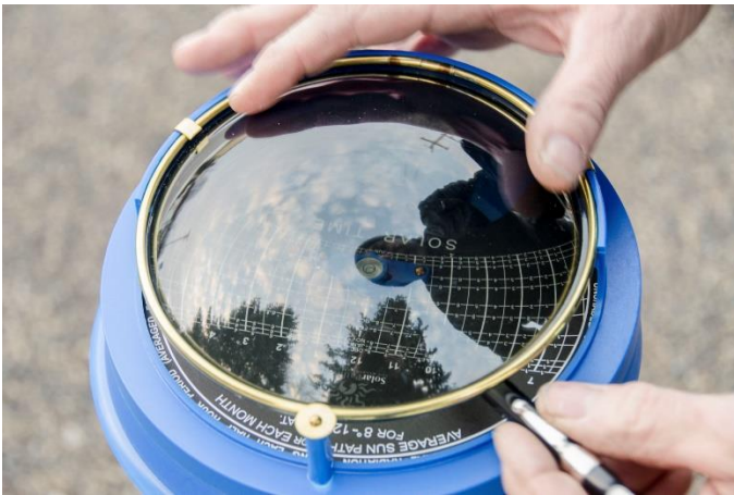
Figure 3.4: Checking for impact of tree shading at one possible solar array location. A white pencil is used to trace the shading on the black paper "Sun Path" diagram that shows the times of shading by month, time of day and the percentage lost to shading. Photo courtesy of FGL/IM-PAHO and SELF.
