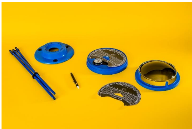
Figure 3.2: Parts of the Solar Pathfinder where reflections seen on the dome can be traced onto a “sun path” diagram to assess shading impact. Photo courtesy of FGL/IM-PAHO and SELF.
