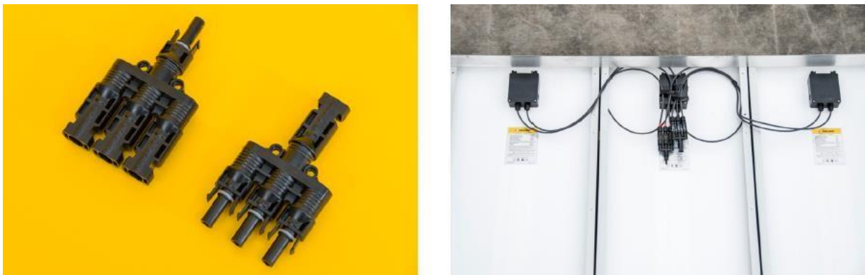
Figure 4.11: Branch connectors for joining three solar modules in parallel with positive (+) output to the left. Note careful wire management has tied loose wires. Photos courtesy of FGL/IM-PAHO and SELF.
