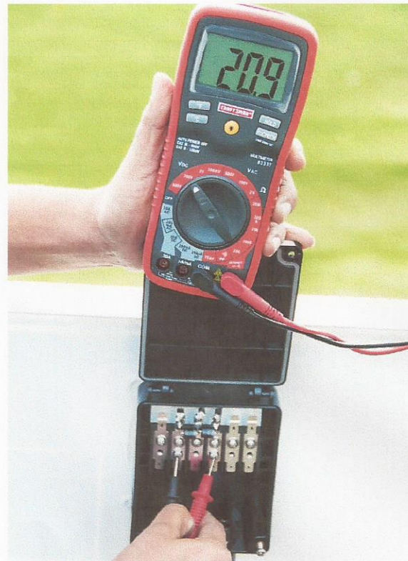
Figure C.5: Measuring solar module open circuit voltage. If the solar module has a standard test rating of 21.8 Voc (at +25°C) its Voc will fall about 1 Volt if the solar module is about 10 °C hotter.
