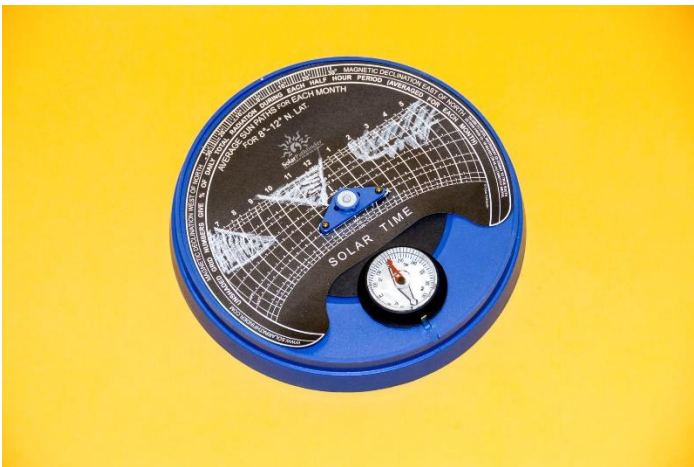
Figure 3.5: Tracing shows too much tree shading for an SDD. Solar array location can be moved to avoid shading. Photo courtesy of FGL/IM-PAHO and SELF.
