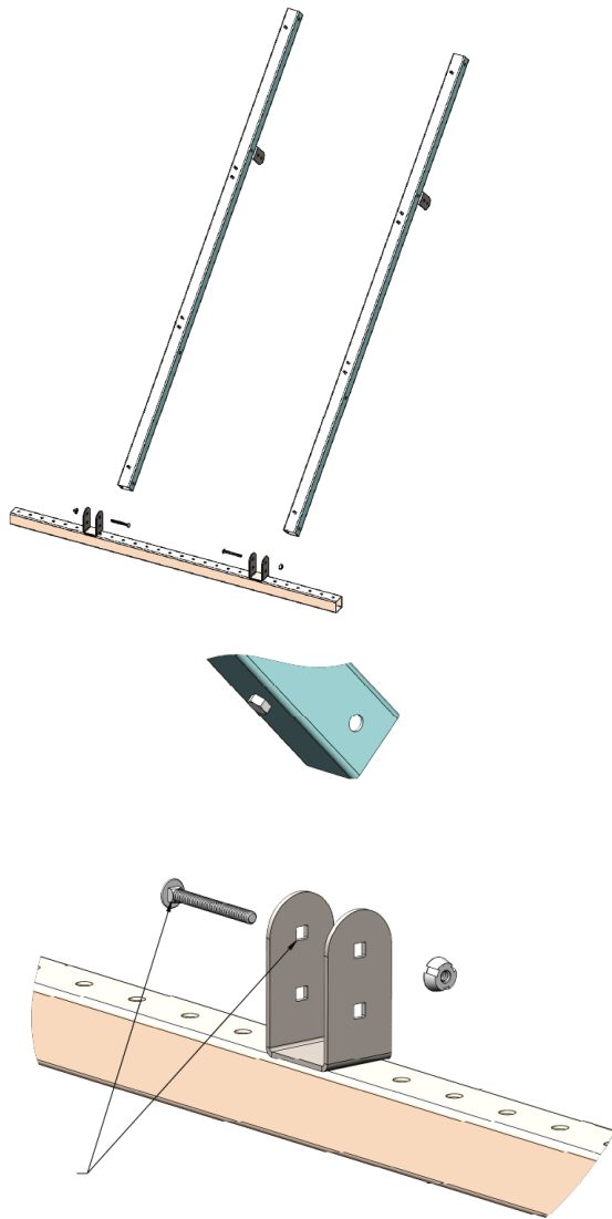
Figure 4.7: Attach module rails. Left: base strut and module rails. Right: carriage bolt detail. Note how square hole prevents carriage bolt from spinning during tightening.
