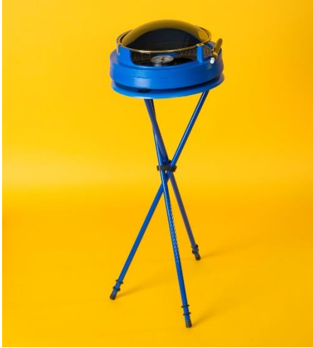
Figure 3.3: Assembled Solar Pathfinder. Photo courtesy of FGL/IM-PAHO and SELF.
