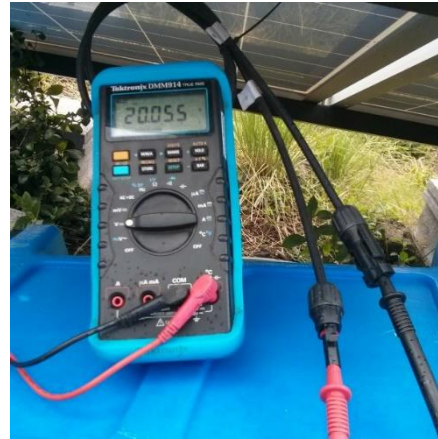
Figure 4.1 Measuring V_{oc} – set multi-meter to measure Volts DC and connect multi-meter to the solar module positive (+) output and negative (-) output. Graphic on left courtesy of FGL/IM-PAHO and SELF.
