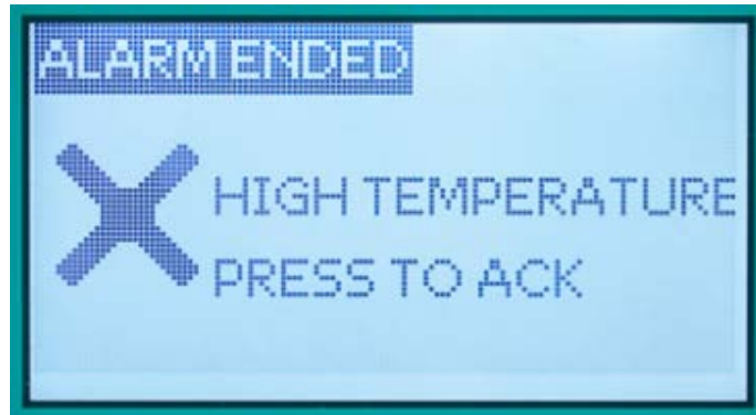
Alarm Ended Screen: Displays information about the most recent un-acknowledged temperature alarm.
